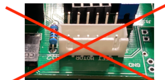
Motor connector Straight Notches outward facing - Wrong
